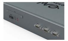
Side A - Detail of CFast slot , serial ports and main power push button switch. APO or ATX selection.
